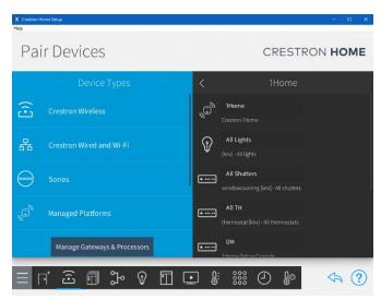
Devices can further be added here to each Room; devices will show with icons per device type with the room name and type identifier.
